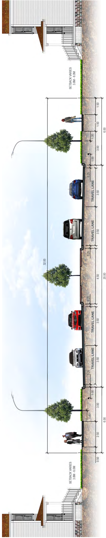
Figure 19 - 32m Divided Collector Roadway Cross-Section at Boulevard.
