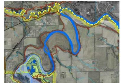
Illustration of a floodplain based on topography and estimated flood elevation.
