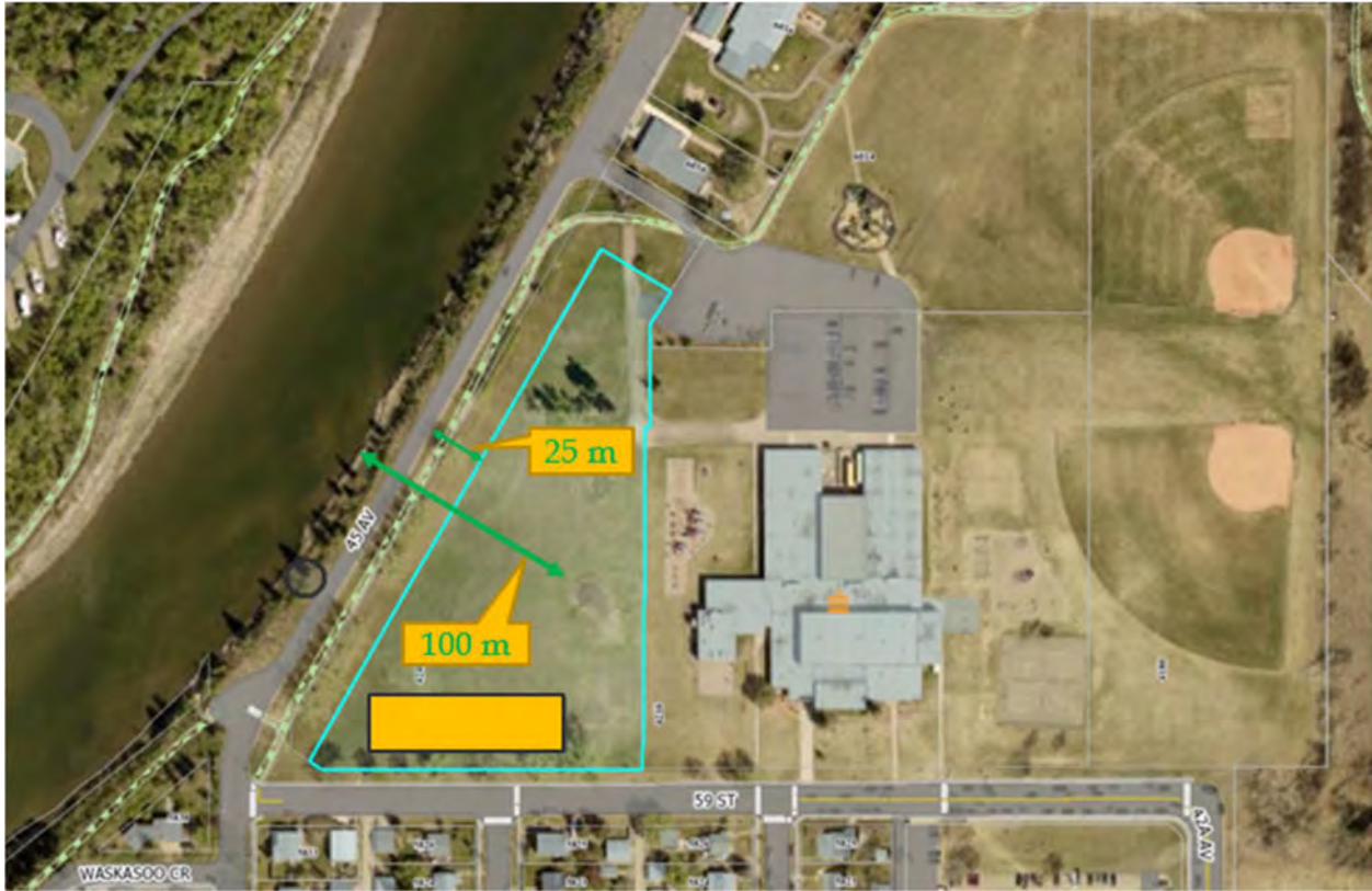
Fig 2: This property lies adjacent to about 250 m of the riparian corridor . The width from waterline to the road varies from 12 to 15 m . In many places there is a little as 4 m between the road and the bank crest. The road is 7.5 m wide and the 3 m wide paved park trail lies within the road allowance. A 15 m municipal reserve separates the property from the road allowance. Note that a 100 m riparian buffer would extend to the base of the play hill near the east side of the property.
