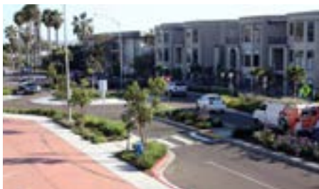
Example of mid-block crossing with bump-outs.
