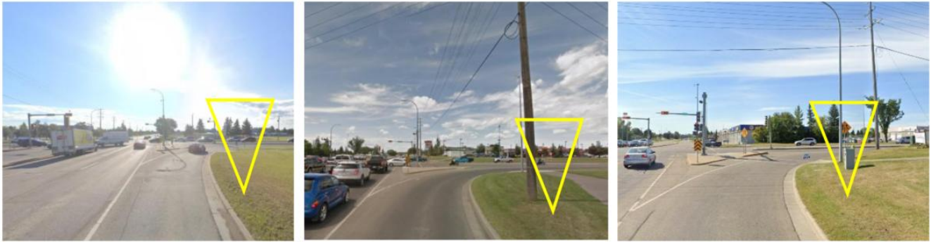
Figure 11: Sightline Restrictions of Signs on the Inside of the Channelized Right Turn Lanes 4
