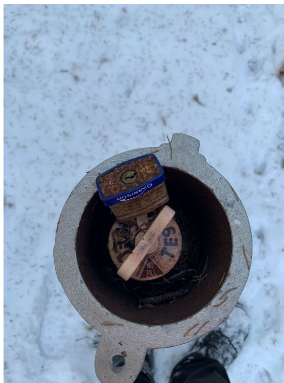
Photo 2: MW-05 missing protective cap
