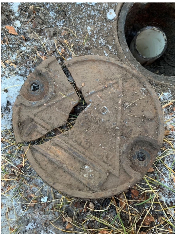
Photo 1: MW-02 broken cap
