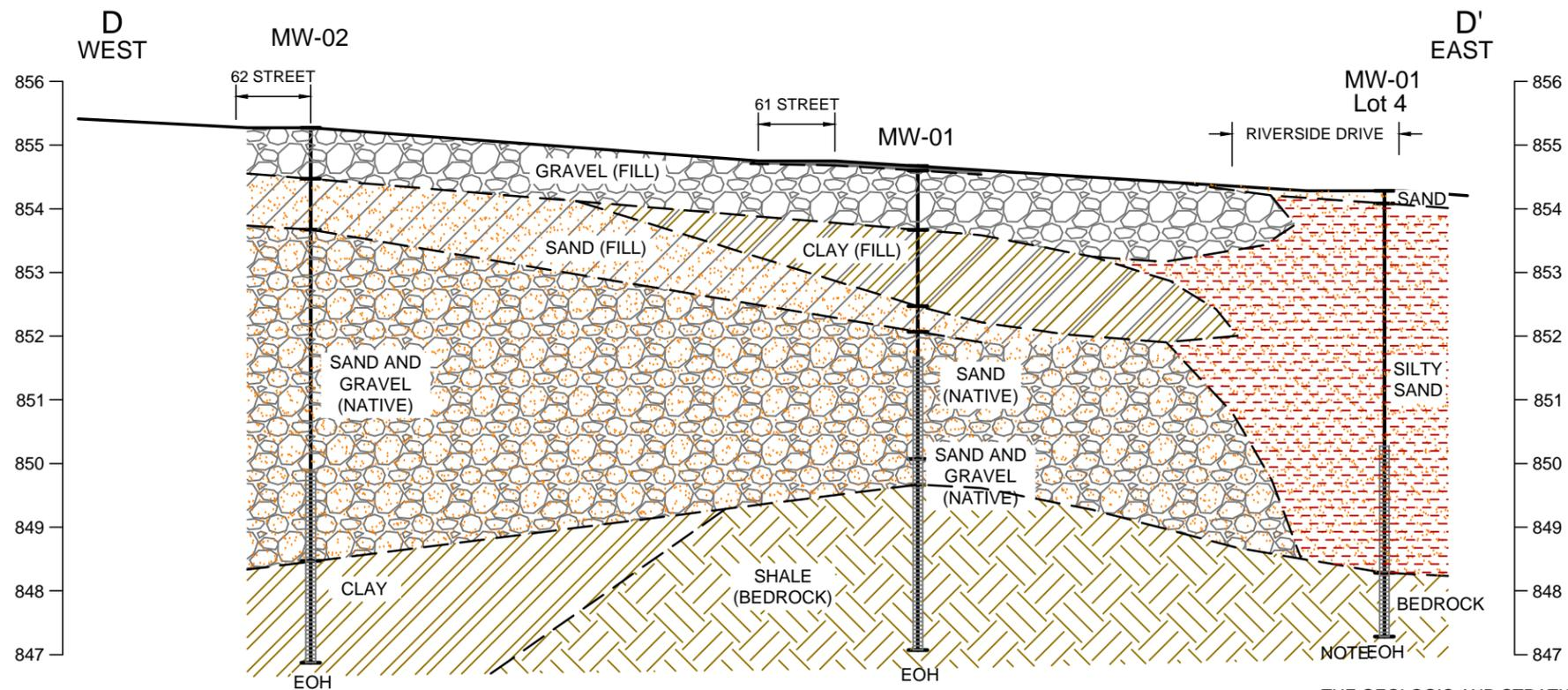
THE GEOLOGIC AND STRATIGRAPHIC SECTIONS SHOWN ON THIS DRAWING ARE INTERPRETED FROM BOREHOLE LOGS. STRATIGRAPHY IS KNOWN WITH CERTAINTY ONLY AT THE BOREHOLE LOCATIONS. ACTUAL STRATIGRAPHY AND GEOLOGIC CONDITIONS BETWEEN BOREHOLES MAY VARY FROM THAT INDICATED ON THIS DRAWING.
