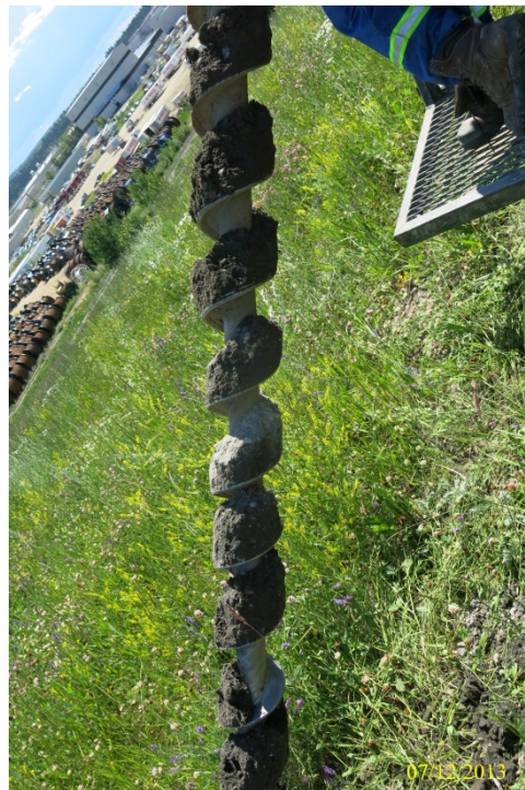
Photograph No. 10: View of MSW on the auger from a depth of 1.5 m to 3.0 m in depth at TH-03.
